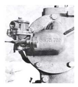
66. Release the lock wire securing the lubricating oil strainer. Lift out the strainer, wash it and blow it dry with compressed air. Re-fit it and lock it with the lock wire. Turn the engine and fit the complete oil strainer.
