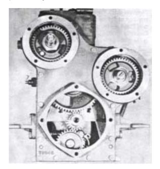
63. Place a new gasket on the water pump and fit it with the two bolts. Make sure that the groove in the pump shaft engages in the flange nut.
