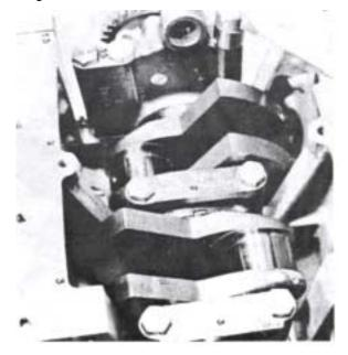
52. Turn the piston rings so that their respective gaps are apart from each other. The piston top is marked with "Front" and should point towards the flywheel. NOTE! Fit the connecting rod which is marked with punch pops nearest the flywheel. Carefully tap the piston downwards through the installation tool with a wooden handle or similar. Place the engine on its side and tighten up the caps. Tightening torque = 50 Nm (5 kpm = 36 lbft). Lock the bolts with the lock washers.
