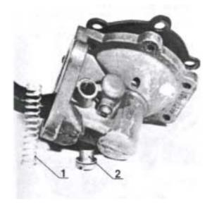
43. Undo the screw 1, and pull out the manual pump lever 2 and replace the spring 3 if in poor condition. NOTE! keep an eye on the rubber seal which is pressed into the body.
