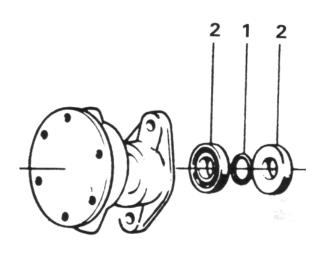
46. Unscrew the bolt and pull the impeller off the shaft. If the sealing rings also have to be replaced, the shaft can be pulled out entirely together with the impeller, after which the bolt can be released.
