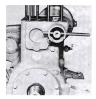
10. Remove the flywheel. Remove the nut and use a puller. The axle is tapered and provided with a key. Use a counterhold when releasing the nut.
