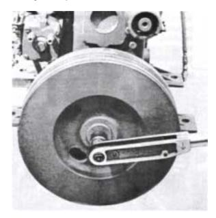
MD6A. Install the stars generator with its bracket. Screw tight the tensioning bar to the engine. Earlier engines have a washer placed between the engine and bracket.
