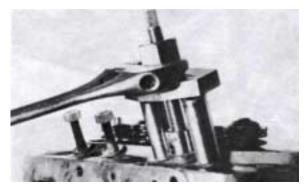
34. Replacing the 0-ring which seals between sleeve and cylinder head.
