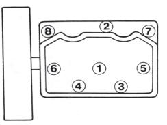
61. Place a new gasket on the inner timing gear cover and fit the outer timing gear casing. Two short bolts are fitted at the bottom. Trim off any part of the gasket which sticks out.
