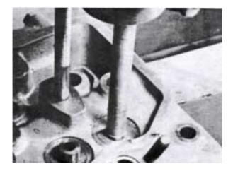
32. Fit new valve guides with tool 884549. Use a press.
