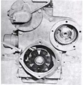
11. Knock out the hand starter pin in the camshaft. Remove the protective cover (2 bolts). NOTE! Scrap the sealing ring and fit a new one.
