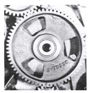
59. Install the fuel injection pump. Use a new gasket. Fit the key on the pump shaft and install the gear wheel. IMPORTANT! The figure must face towards the figure on the intermediate gear. Tighten up the gear wheel with the nut which also functions as a flange for the water pump. Tightening torque = 60 Nm (6 kpm = 43 lbftf). Use a counterhold.
