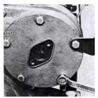
8. Remove the nut which drives the water pump. Use the flywheel as a counterhold. Remove the fuel injection pump and the gear wheel.
