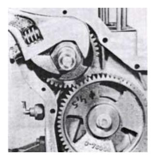
15. Remove the bolt for the intermediate gear. Discard the sealing washer 1 under the bolt. Pull off the intermediate gear.
