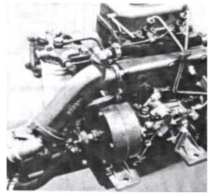
Fill the engine and reverse gear with oil. Concerning the oil quantity and quality, see under "Technical Data".
