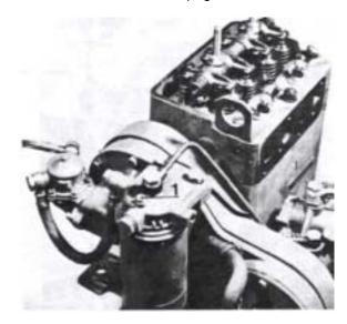
69. Fit the key for the flywheel and push on the flywheel. Fit the thick washer and tighten up the flywheel with the nut. Tightening torque = 180 Nm (18 kpm = 130 lbftf). Use a counterhold through the flywheel.
