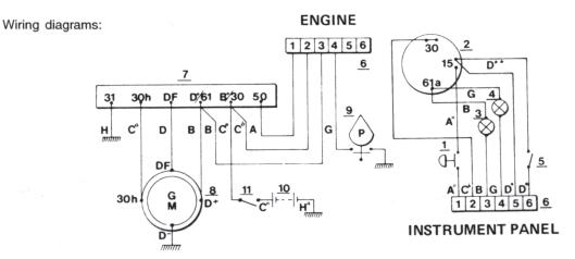
Fig. 82 Wiring diagram for the MD6A with start-generator (no rev counter and temp. gauge)
