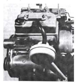
79. Fit the key in the crankshaft. Heat the flange and fit it on the shaft. Tighten it up with the bolt and the thick washer. Tightening torque: 80 Nm (8 kpm = 57 lbftf). Bend down the thin washer over the bolt head. Fit the rubber damper.
