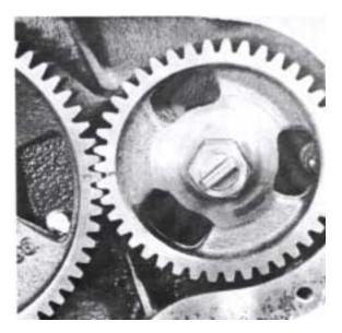
58. Place the large flat washer on the intermediate gear with the bevel facing outwards, and thereafter the steel-rubber washer 1. Tighten with the bolt. NOTE! On earlier engines a plastic washer is used. This must be scrapped and replaced by the steel-rubber one.
