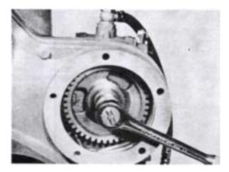
9. Remove the timing gear cover. NOTE! The small round cover on which the fuel pump is mounted has bolts with 3 different lengths. The bolts for the large casing has two lengths. The two bottom bolts are shorter than the others. Carefully lever loose the timing gear casing from its guide pins. Discard the gasket.
