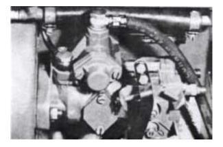
7. b. (CAV pump) Disconnect the pipe from the fuel filter and remove the nuts for the fuel injection pump.
