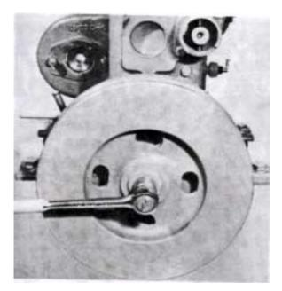
12. Remove the front cover behind the flywheel (11 bolts). Note the guide pins. Carefully tap all round. Replace the gasket and the sealing ring.
