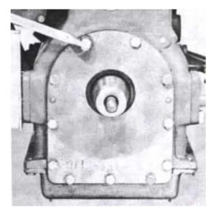
68. Fit the rocker arm, fuel filter and fuel lines. NOTE! Replace the fine filter insert (see page 25, Point B) by turning the hex head in the bottom of the container. When the installation of the engine is completed, bleed the fuel system through the bleeder screw 1. See more detailed instructions about this on page 25, Point B.
