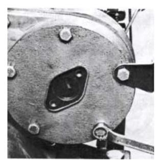
64. Fit the cover with new gasket over the camshaft end. NOTE! The bolts have three different lengths. The Fig. below shows where they are placed.
